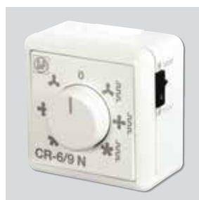
CR-6/9 2 Power remote selector and 3 speed fitted with the fan to control up to 5 units in series of the A/H models (ambient and hot air) . LxWxH (mm): 88x47x88
